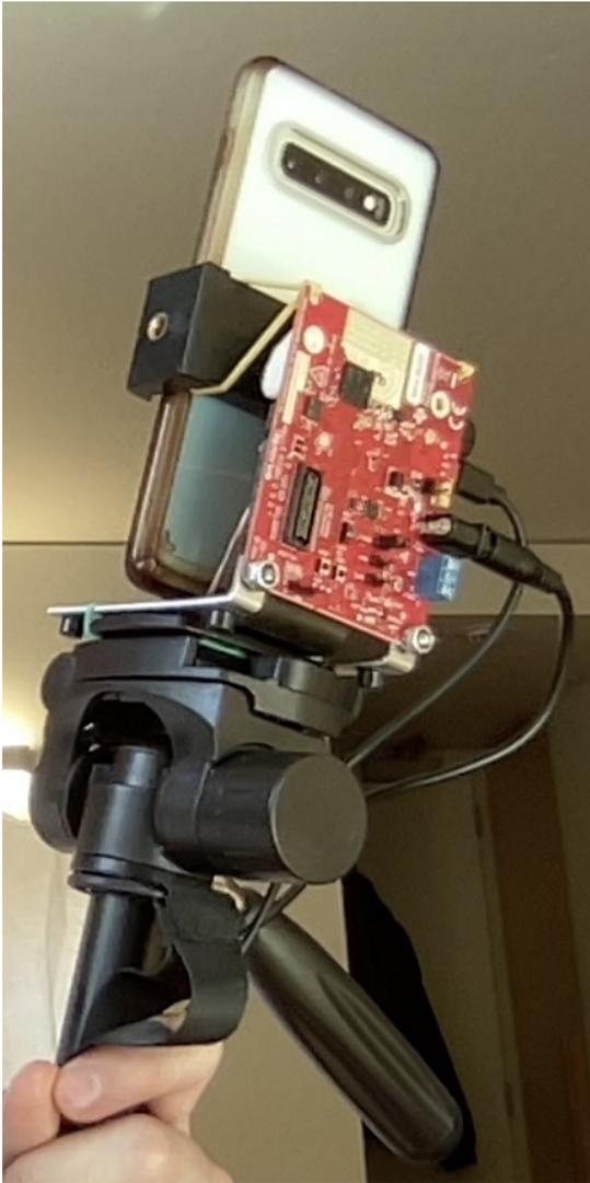
Figure 5.2: The final constructed device to be used for data collection, using the IWR1443BOOST evaluation board (red circuit board), and an Android phone.
